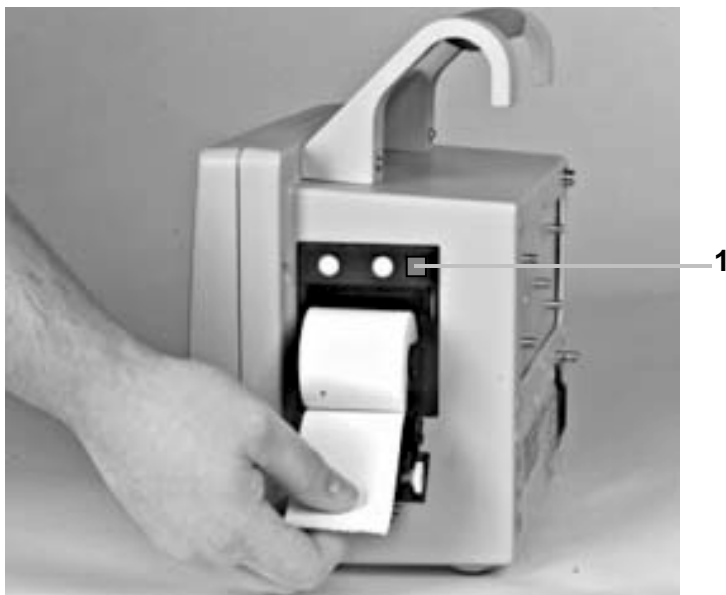
Figure 29: Loading Thermal Paper in Printer
